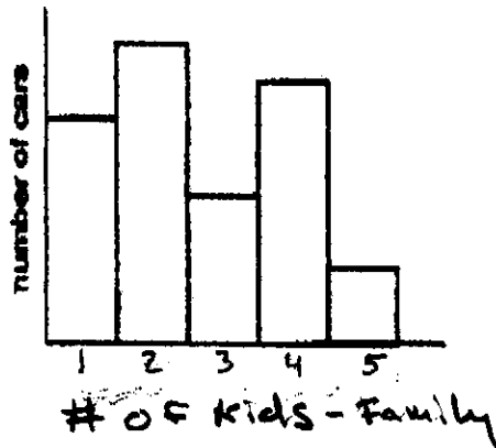
Ex. Histogram. Frequency for "Quantitative Data" best for discrete & not overlapping information
